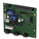
The EV-CC-AC1-M3-CC-SER-PCB charging controller as a PCB for charging electric vehicles on a 3-phase AC power grid according to IEC 61851-1, Mode 3. Optimized for charging stations with permanently mounted Vehicle Connector. All charging functions and comprehensive configuration settings are already integrated.
